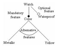
Figure 2 FODA-style feature diagram
